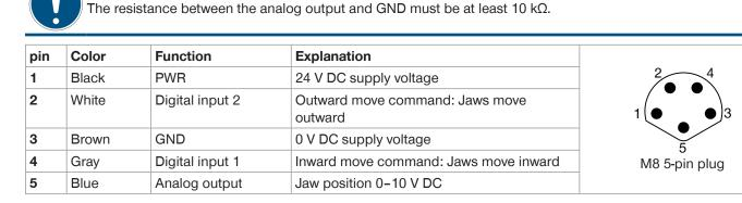
The inputs of the product are configured for 24 V DC PNP outputs of the control system.
