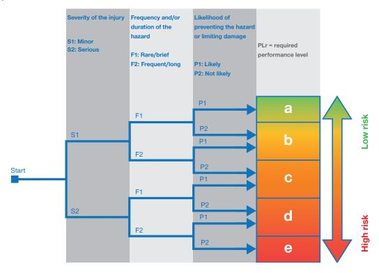
The EN ISO 13849-1 also uses a risk graph to determine the required safety level **PLr**. Parameters S, F and P are used to determine the severity of the risk.
